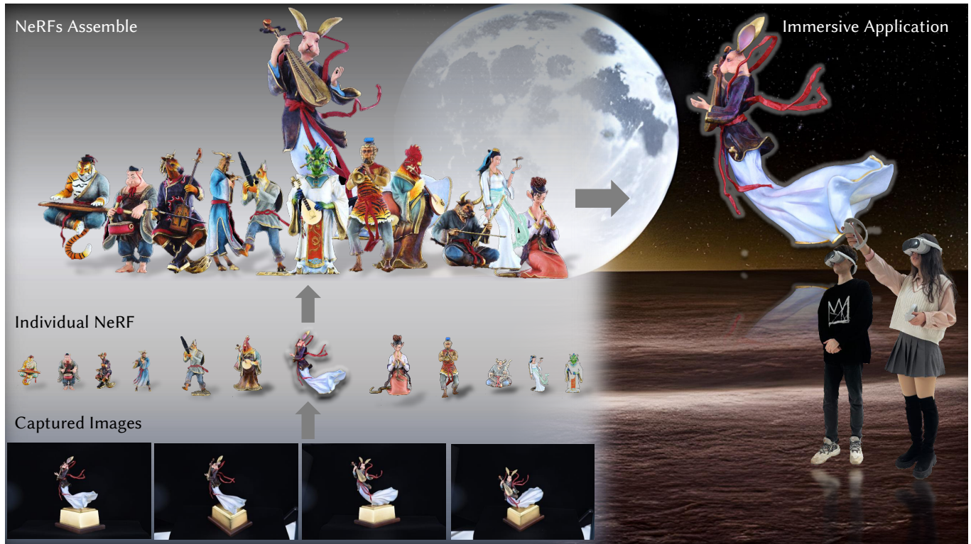
Fig. 1. Demonstration of our NEPHELE platform. We present NEPHELE, a neural platform for highly realistic cloud radiance rendering. Our approach represents the objects, e.g., the Chinese zodiac , as i-NOLFs for ultra-fast neural radiance rendering. With a tailored task scheduler, NEPHELE allows for utilizing the power of multiple GPUs to render a complex scene composed of many neural assets which cannot be achieved by a single GPU. NEPHELE further distributes the photo-realistic radiance renderings to the clients so that everyone can easily access the shareable neural assets on the cloud via various devices such as VR headsets and mobiles.
